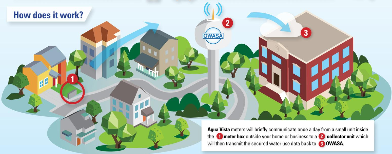
**Agua Vista** meters will briefly communicate once a day from a small unit inside the **1** meter box outside your home or business to a **2** collector unit which will then transmit the secured water use data back to **3** OWASA.
